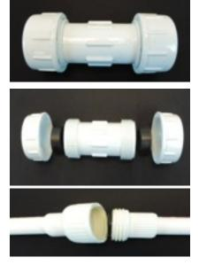
above, they are used to join two pipes together. However, unions have some special properties that allow them to be taken apart for repairs or for mobility. Once the pipes are connected to the two halfs of the union, they screw together (without the need for the pipes to turn) and include a washer to provide a water-tight seal.
