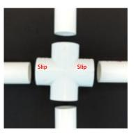
when using crosses in plumbing applications as they can generate large amounts of stress on the connecting pipes as temperature changes occur. Manifold crosses are primarily used in fire sprinkler and irrigation systems, allowing the "main" line to be connected on a slip-to-slip basis while allowing the "cross" connections to the "manifold" line to be threaded connections.
