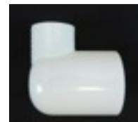
One configuration of the 90 degree reducing ell is the **Schedule 40 “90° reducing slip x slip elbow”**. This 90° elbow allows for two different size pipes to be connected at a 90° angle by cementing both pipes into the elbow. Both pipe ends are glued into the ell, forming a 90° turn or joint comprised of two different size pipes.
