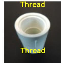
If one pipe has a thread on it and the other end is smooth or has no thread, you will need a “**SLIP/FIPT coupling**”; more commonly called a **female adapter**. These couplings or “adapters” have a slip end on one side that your pipe glues into, and a thread on the other side that accepts the male pipe thread. The fitting is normally screwed onto the threaded pipe first and then cemented or “glued” onto the pipe with no thread to complete the fitting.
