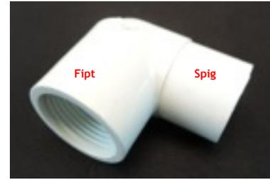
Yet another configuration of the 90° street elbow is the **Schedule 40 “90° street mipt x fipt elbow”**. This fitting has a female (fipt) “street” or “spigot” side that fits into another fitting, with a male thread (mipt) fitting that accepts the incoming pipe. So for example, a 3/4” 90° street mipt x fipt elbow would actually screw into a 3/4” fitting and then a 3/4” male pipe would screw into it.
