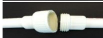
above, they are used to join two pipes together. However, unions have some special properties that allow them to be taken apart for repairs or for mobility. Once the pipes are connected to the two halves of the union, they screw together (without the need for the pipes to turn) and include a washer to provide a water-tight seal.
