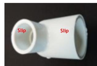
Another configuration of the 90 degree reducing elbow is the **Schedule 40 “90° reducing slip x fipt elbow”**. Using this elbow allows the user to connect two different size pipes at a 90° angle when one pipe has a smooth exterior and the other has a male pipe thread. The nomenclature can be a little tricky on these fittings.
