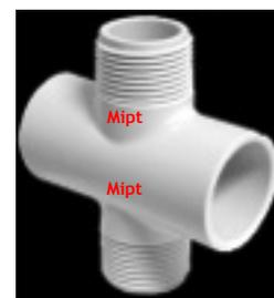
when using crosses in plumbing applications as they can generate large amounts of stress on the connecting pipes as temperature changes occur. Manifold crosses are primarily used in fire sprinkler and irrigation systems, allowing the “main” line to be connected on a slip-to-slip basis while allowing the “cross” connections to the “manifold” line to be threaded connections.
