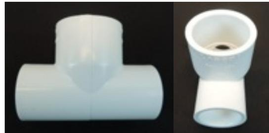
Another specialty tee is called the “**manifold tee**”. Manifold tees are primarily used in irrigation systems, allowing the “main” line to be connected on a slip-to-slip basis while allowing a threaded connection to the “manifold” line. The two opposite ends of the manifold tee have slip fittings while the “top” of the tee has a male thread fitting.
