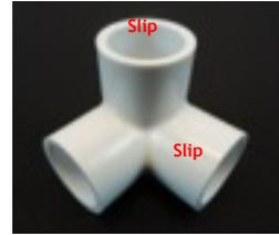
Side Out elbows with slip socket fittings on all three outlets are the most common, and are known as **Schedule 40”Slip Side Out Elbows”**. All the three smooth-end pipes coming into the fitting at right angles are all cemented into the fitting for a secure connection. All three incoming pipes are equal in size.
