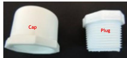
**Schedule 40 Slip Caps** are used when a more permanent cap is needed for your project, or where a threaded solution is either not practical or available. Slip caps solvent weld or cement onto a smooth Schedule 40 pipe for a secure connection. They must be cut off if they need to be removed.
