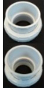
If one pipe has a thread on it and the other end has no thread, you will use a “**FIPT/SLIP Union**”. These unions have a slip end on one side that your pipe glues into, and a female thread end on the other side that accepts the male pipe thread from the pipe. Once the union sections are connected to the pipes, the union is screwed together to form the joint.
