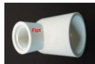
The first size stated is the “slip” size and the second size stated is the “fipt” size. An example would be our 2” x 1” 90° reducing slip x fipt elbow. You would glue a 2” smooth pipe into this end and turn or screw a 1” male threaded pipe into the other end.
