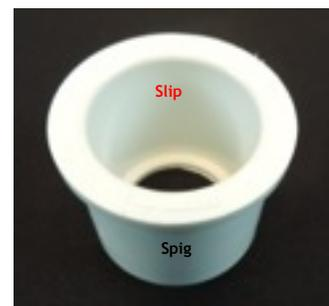
Schedule 40 spig x slip reducer bushing would work like this - the bushing would be glued into a fitting that accepts a smooth 2" pipe or fitting. Then a 1" smooth end pipe would be cemented into the bushing, allowing the 1" pipe to fit into the 2" pipe.
