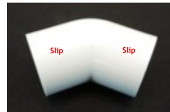
At times, the two pipes that you need to join form a 22.5 degree angle or turn. If both ends of your pipe have smooth ends, you would use a 22.5° slip elbow. **Schedule 40 PVC 22.5° ells** are designed to turn the flow of a liquid at a 22.5-degree angle. Both pipe ends are glued into the ell, forming a 22.5° turn or joint.
